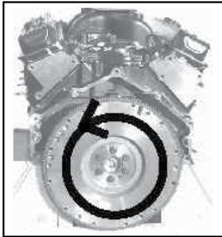
If your FLYWHEEL turns counter clockwise you have LEFT HAND engine rotation
